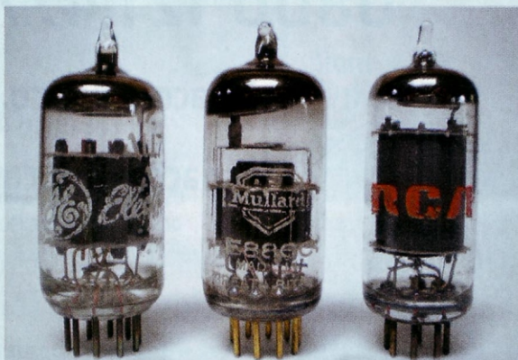
ABOVE: 12AU7 (ECC82) double triode from General Electric's 12A...7 series (left); Mullard E88CC double triode from 1958 (middle); RCA 6BJ6 pentode (right)
