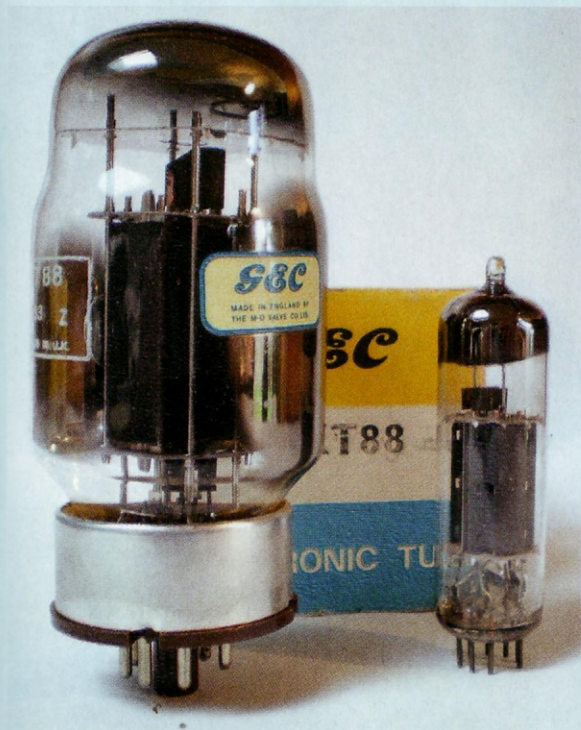
BELOW: Little and large – two popular 1950s power valves in the form of a GEC KT88 beam tetrode with box (left) and an EL84 output pentode
